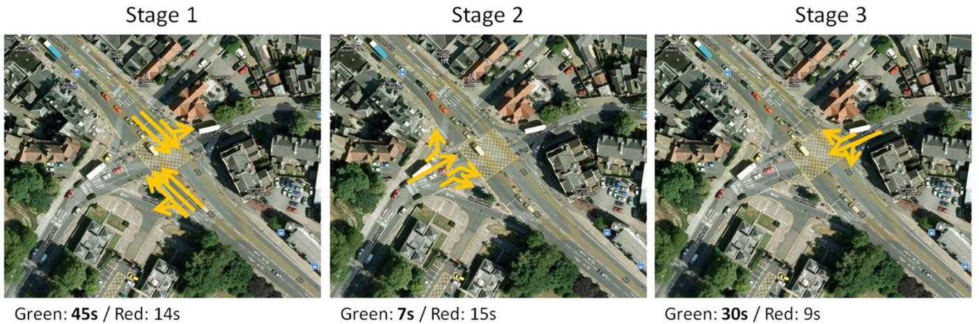
Figure 4. Traffic light signal stages with their default timings for AM (morning) and inter-peak periods, for one junction on the A6 London Road, as optimised in this work. (Background image source: Google Earth, Infoterra)
