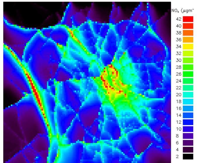
Figure 2. Example of Airviro nowcast (6<sup>th</sup> Oct. 2011, 09:00) as a map of  $\text{NO}_2$  concentrations over the city of Leicester, UK, with a stretch of the M1 motorway (left).
