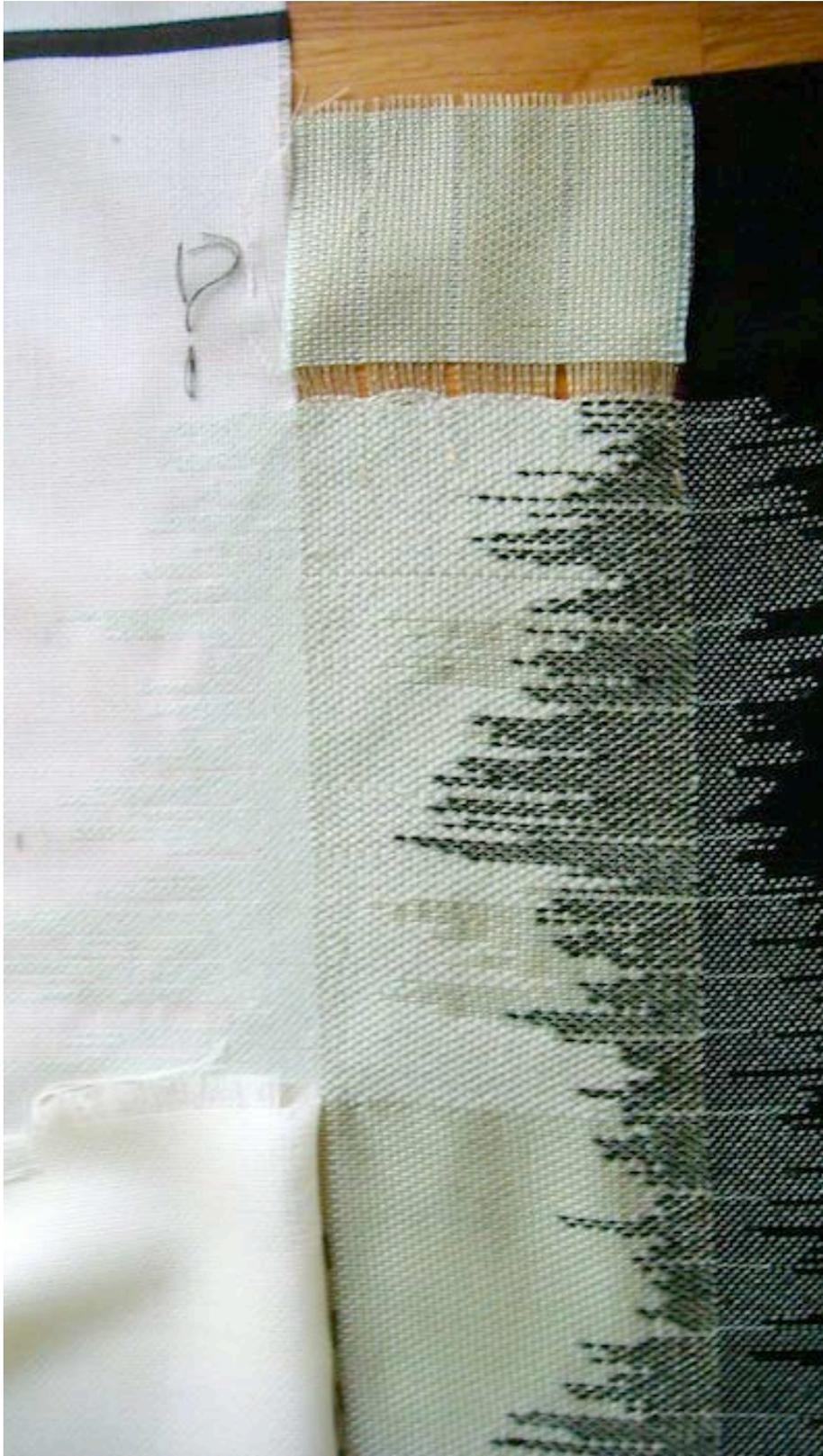
**Figure 2 The process of hand-weaving the seam.**
