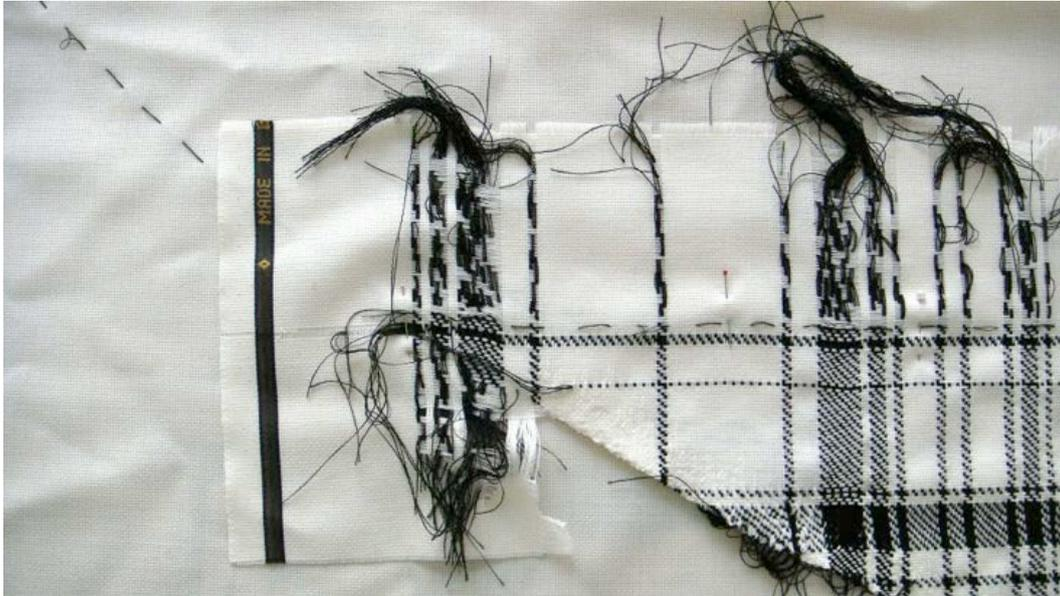
**Figure 7** The process of hand-weaving the seam.
