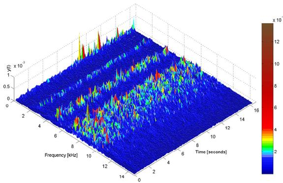
Figure 1: Autonomous helicopter’s intrinsic sound spectrum from test flight 3
