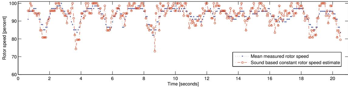
(b) Sound based constant rotor speed estimation
