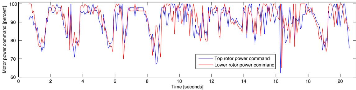
(a) Motor power command to both rotors
