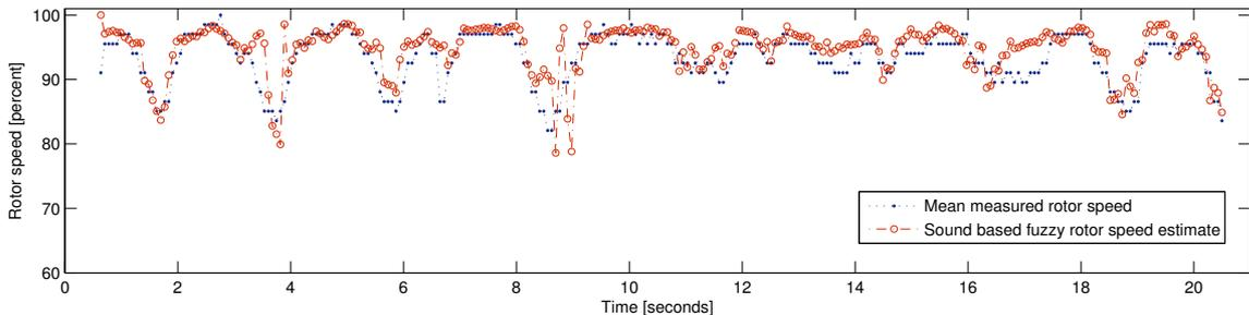
(c) Sound based fuzzy rotor speed estimation
