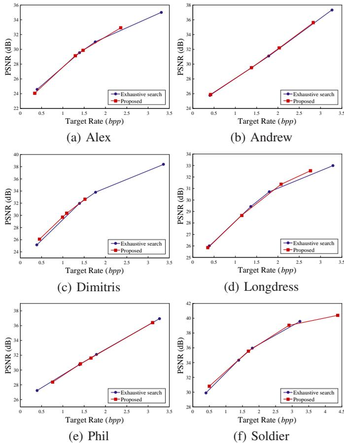
Fig. 8. PSNR vs. target bitrate for the proposed algorithm and exhaustive search.
