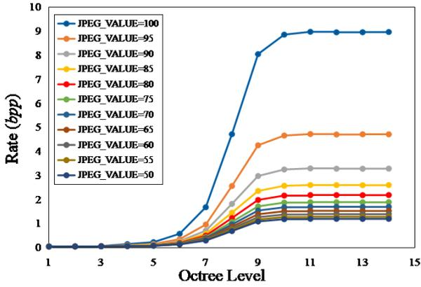
Fig. 1. Relationship between the bit rates, the maximum octree levels, and the JPEG\_VALUES for the *Alex* point cloud set.
